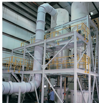
Dual stage HCl scrubber with fiberglass columns and catwalks.
