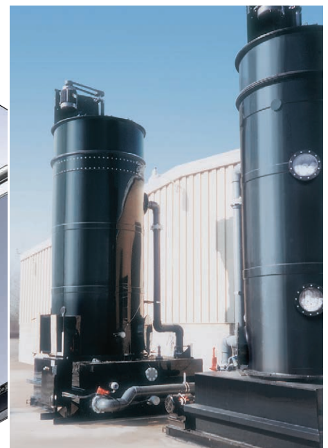
8,000 cfm VTB units constructed of black polypropylene ready to ship.
