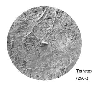
Tetratex® PTFE membrane laminated to needled 16 oz. polyester is a high efficiency media used in pulse jet baghouse dust collectors. This material delivers superior dust cake release and high filtration efficiency in applications with demanding emissions standards. This material is strong, with high resistance to acids and alkalies, and good for applications up to 275° F.
