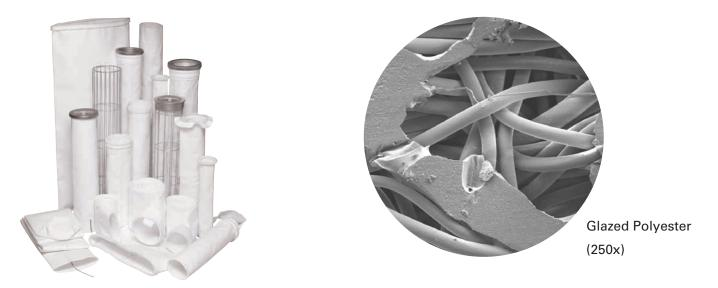
Needled 16 oz. glazed polyester felt is a versatile filtration media used in pulse jet baghouse dust collectors. The glazing process provides a better dust cake release by melting the outermost fibers and smearing them to create a smooth, high sheen surface. This material is strong, abrasion and chemical resistant and good for applications up to 275° F.
