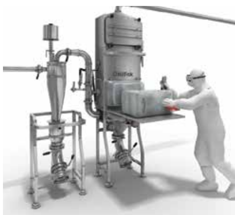
SAFE HEPA FILTER REPLACEMENT
