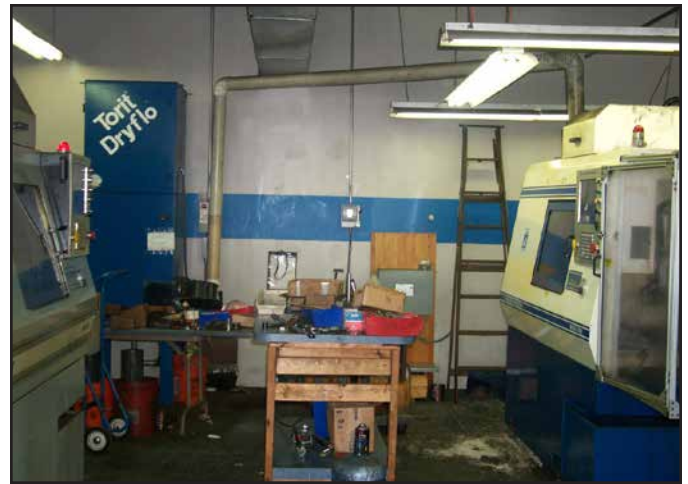
AL) Example of PVC pipe connecting a Donaldson Torit Dryflo mist collector to a machining center
