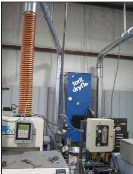
AK) Clamp together ducting (Donaldson Torit Easy Duct™) used from the mist collector, with a short piece of flex hose to connect to the application
