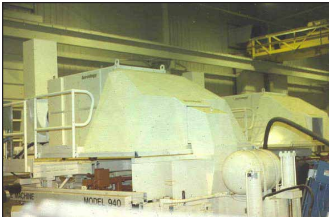
Z) Canopy-style hood on die cast mist collector, on casters, to roll out of the way for maintenance
