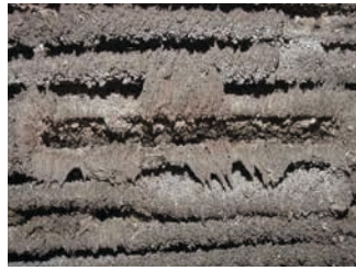
L) A vee-bag after collecting die casting mist
