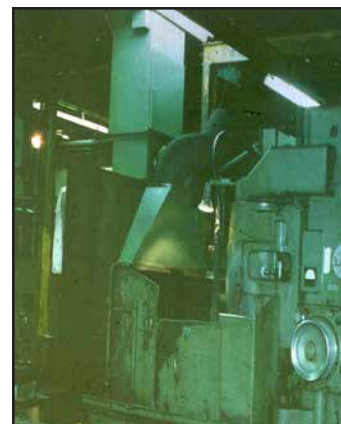
Y) 30-inch Blanchard with hood and mist collector
