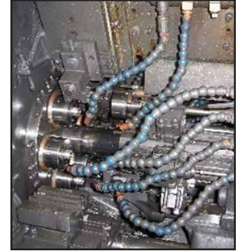
F) Internals of Acme Gridley Screw Machine
