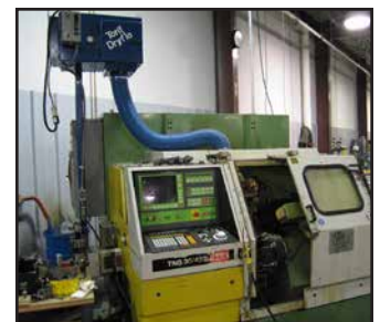
AN) Poor installation of Flex Hose (starting to sag)
