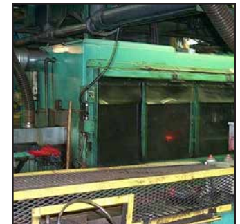
O) Oil quench of steel springs
