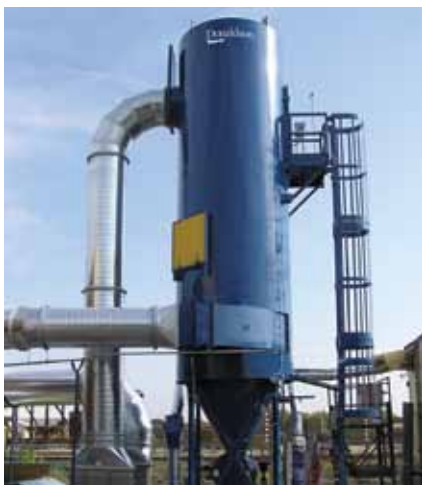
RF DUST COLLECTOR
