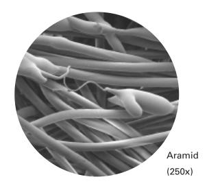
Needled 14 oz. aramid felt is a high temperature filtration media used in pulse jet baghouse dust collectors. This material performs well in dry, high heat applications. It is strong, abrasion resistant and good for applications up to 400° F.
