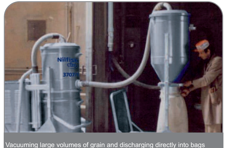
Vacuuming large volumes of grain and discharging directly into bags
