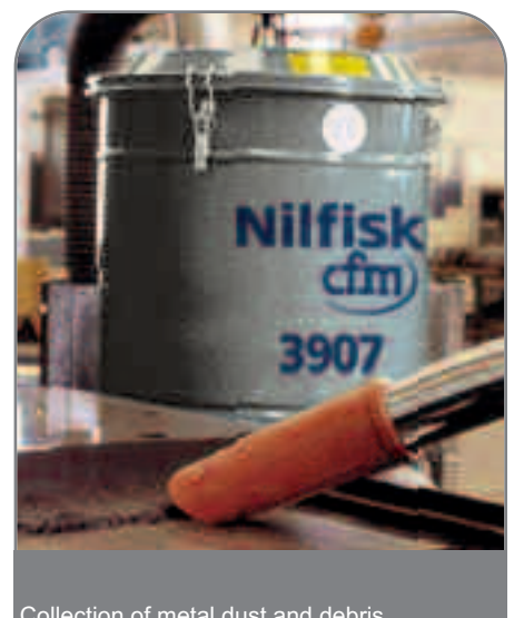
Collection of metal dust and debris
