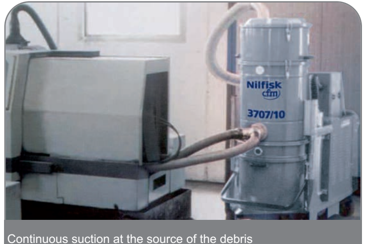
Continuous suction at the source of the debris
