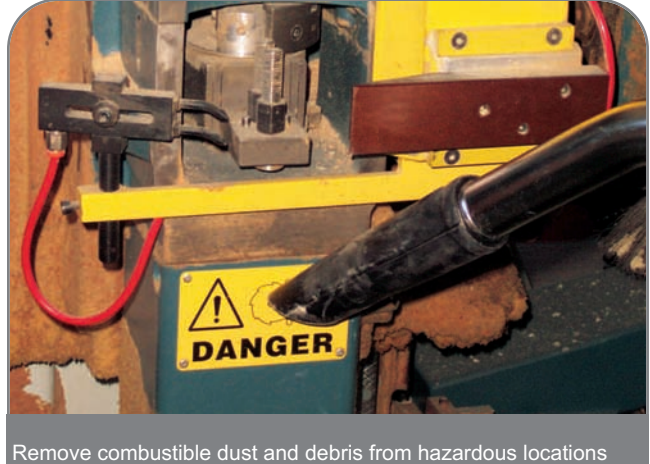
Remove combustible dust and debris from hazardous locations
