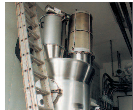
Q-Rohr® installed in a milk powder factory
