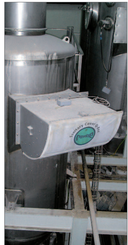
Q-Box II application in the food industry: the sanitary cover protects the exterior of the Q-Box II; keeping it clean from the outside
