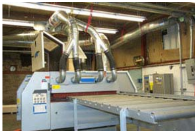
There are several dust pick-up points on this automated saw, all ducting into the Donaldson Torit RFW dust collector.
